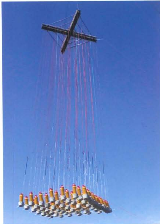
FIGURE 4.15 Each charge was suspended with two ropes: The lower was destroyed in the blast, while the upper could be reused.
