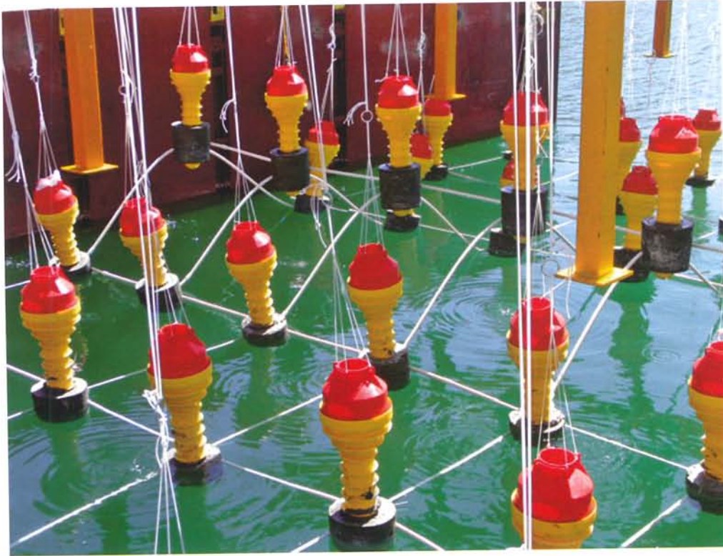
FIGURE 4.13 Testing the flexibility of the PVC-pipe grid, which kept the charges at proper spacing.
