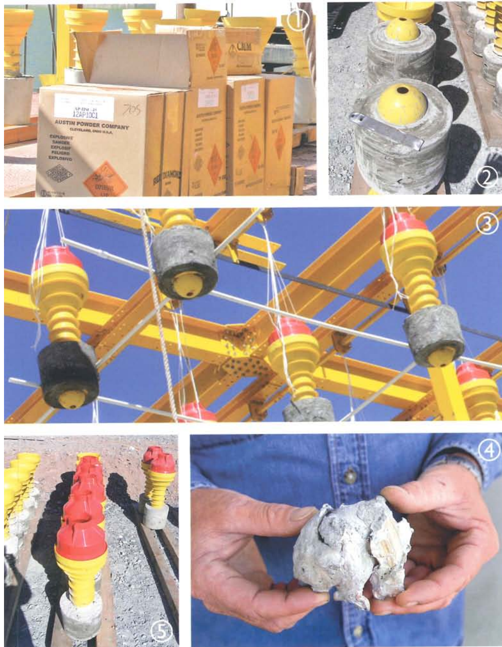
FIGURE 4.11 Shaped charges. ① Composition B explosive. ② Concrete ballast. ③ Charges arranged on a test frame. ④ Part of a slug following detonation. ⑤ Shaped charge shells.
