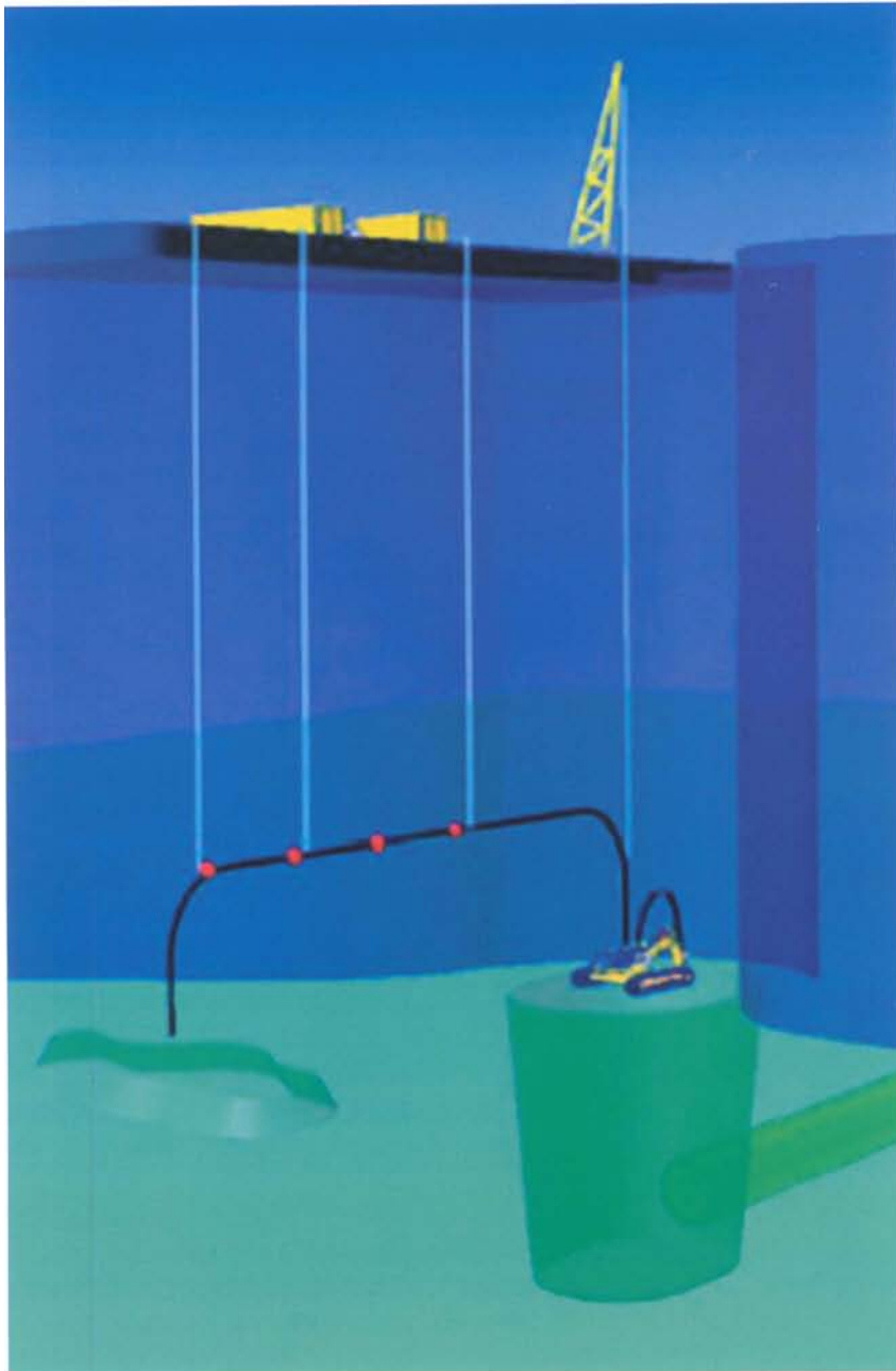
FIGURE 4.7 Another excavation method considered used virtual reality techniques to control a first-of-its-kind excavator equipped with a crusher head and airlift system to transport excavated material.
